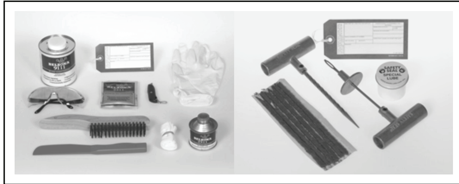
Figure 6-10. Tire patch materials and tire plug kit
